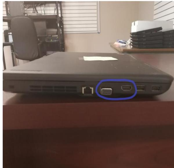
3. You will need to plug one end of the VGA cable into the laptop and the other end into the box on the wall that goes to your projector.
